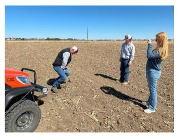
Soil samples are taken throughout the field – one sample for every 8 acres. Sample locations are determined by computer software. These samples are used to verify the soil fertility information collected by the SoilOptix Sensor
